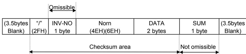
Norn (1 byte) : Communication error command ... This command is also used for a check when the inverter is tripped.
