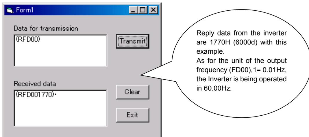
2)Arrangement of the control on the form
