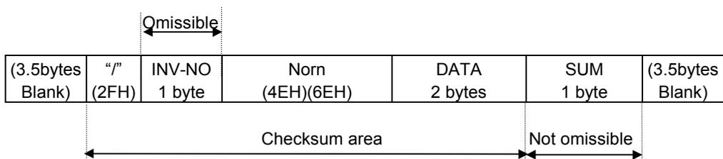
"N" or "n" (1 byte) : Communication error command. Also for check during an inverter trip (includes standing by for retrying and trip holding). "4EH (N)" when normal, "6EH (n)" during an inverter trip.
