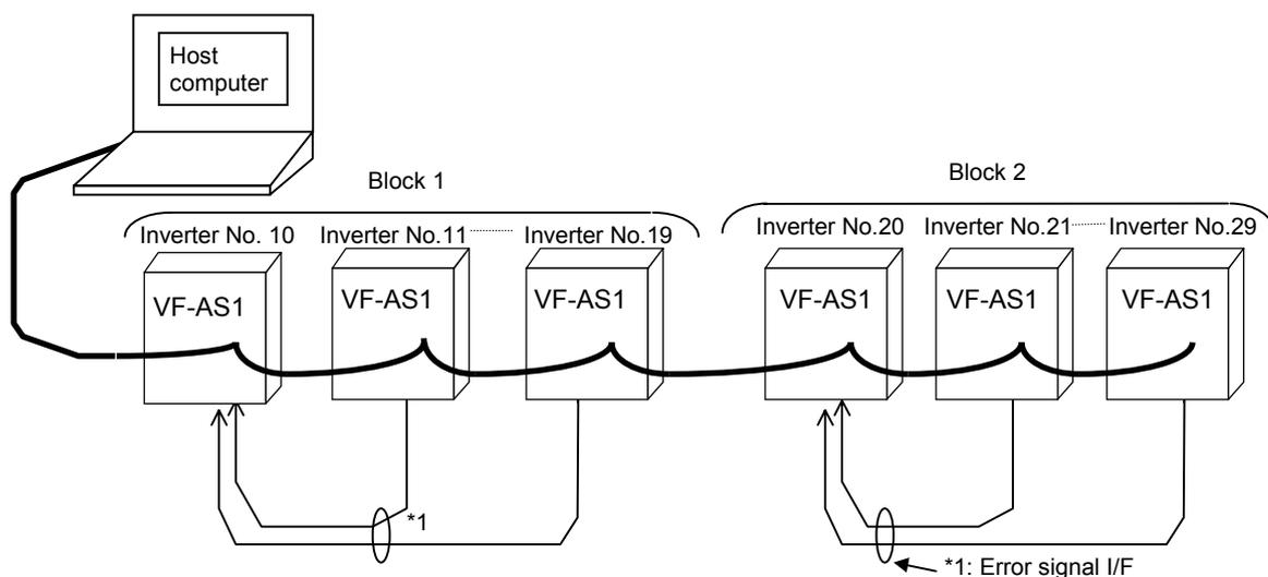
In broadcast communication, only the representative inverter in each block returns data to the host computer. However, you can make the representative inverter in each block report the occurrence of a problem in the block. To do so, follow these steps.
